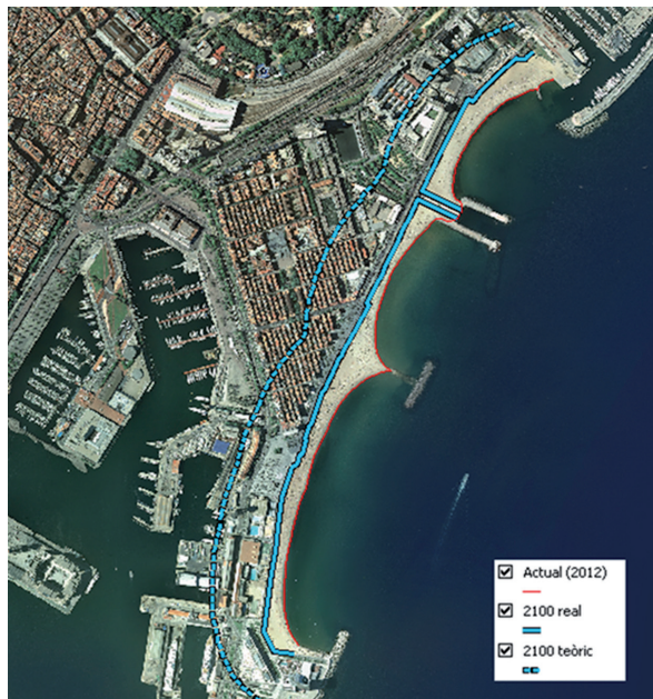
Figure 13. Changes in the edge of the Barceloneta beach, caused by rising sea levels, with a sandy beach (the theoretical case) and rigid infrastructures (the real case).
