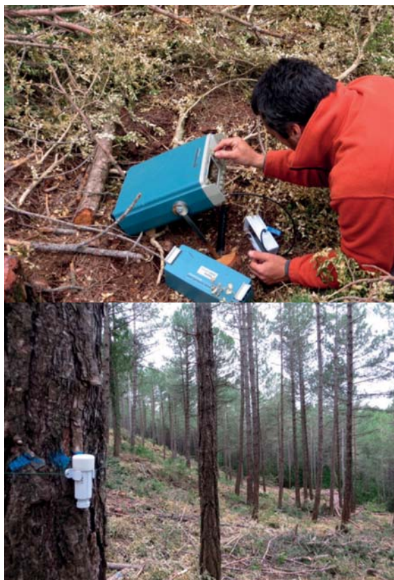
Segre Measuring water soil content and Segre Pilot in forests
